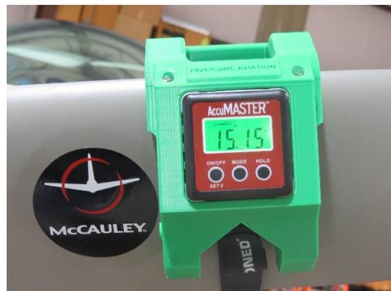
15. Continue to rotate the propeller in the direction of forward rotation until the inclinometer reads the divided by 2 number.
