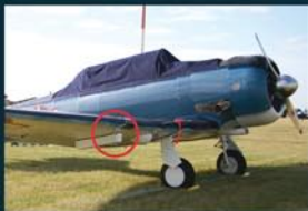
TYPICAL AOA PROBE LOCATION
