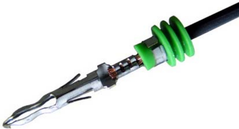
Seal loaded on stripped wire (wire stripped 5.0mm or 3/16")
