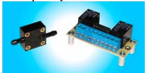
Airspeed Relay - used for: Flap Deployment Protection and Automatic Speed Adjust for Elev. Trim Motors
