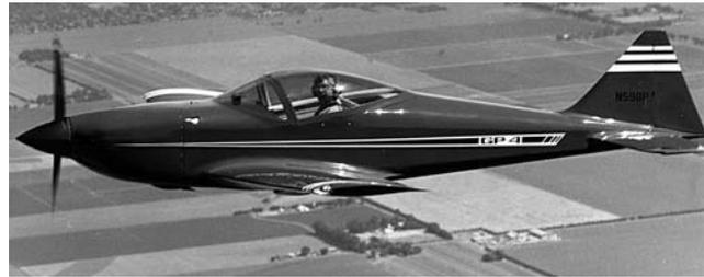
Designed by George Pereira, the GP-4 is a high performance two place side-by-side kit aircraft which is a fast, efficient cross country performer. Construction is primarily of wood and steel. The GP-4 is becoming the choice of many builders seeking a solid, traditionally constructed scratch built aircraft.
