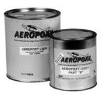
Aeropoxy Light, a modification of the ES6279 adhesive system, is a 2-component paste epoxy patching and filler compound for foam, wood, fiberglass and other surfaces. The mixed consistency of this system is very smooth and creamy, so it spreads easily, and can be spliced to a feather edge without separation. It is a thixotropic, non-sag material that will remain in place in thick sections, even when applied upside down! The resin and hardener of this system are color coded for easy mix-
