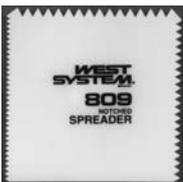
This plastic spreader is excellent for spreading epoxy at a steady rate to provide an even surface. Measures 4" x 4" and is notched on three sides in increments of 1/8", 3/16", 1/4".
