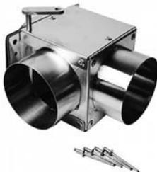
P/N DL-005 - This box is identical to the deluxe stainless steel cabin heat box, except that the inlet and outlet are 2 1/2" OD so that this box can be used when the builder wants to use 2 1/2" scat tubing throughout the project. (This box was used on the Cirrus SR20 certified aircraft. The SR20 now uses the DL-008 box listed below.) Weight is 6.3 ounces. ....P/N 08-04015.....\$163.85
