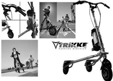
Tribred Pon-e: transportation/fitness/joyride all in one vehicle. Lightweight high-performance aluminum frame with lithium battery power. Specifications: • Color: green or silver • WT: 38 Lbs • 10" air tire brushless • Geared hub motor 250W • Free wheel clutch • Removable 36V - 9Ah Lithium-Ion battery with Panasonic cells • Features key & lock • 2 Modes: ECONO max 12 mph / EXPRESS max 17 mph.
