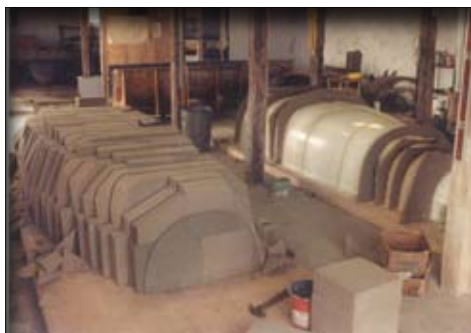
The fuselage plug started with bonded foam which was shaped into a core.
