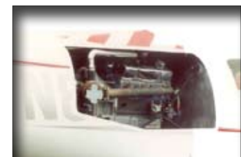
The (in)famous V-8 auto engine installation...before the fire.
