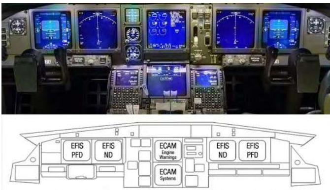
Figure 1-6. Boeing 777 Electronic instrument system has 6 LCD Displays.
