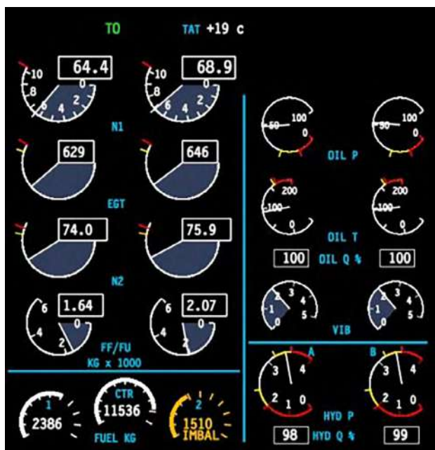
Figure 1-9. EICAS engine display format.
