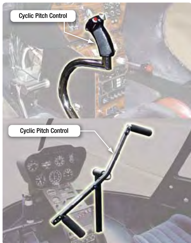
Figure 1-43. The cyclic pitch control may be mounted vertically between the pilot's knees or on a teetering bar from a single cyclic located in the center of the helicopter. The cyclic can pivot in all directions.
