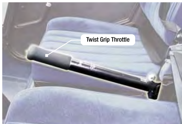
Figure 1-42. A twist grip throttle is usually mounted on the end of the collective lever. The throttles on some turbine helicopters are mounted on the overhead panel or on the floor in the cockpit.
