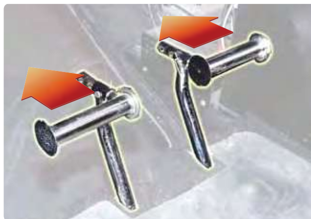
Figure 1-45. Antitorque pedals compensate for changes in torque and control heading in a hover.
