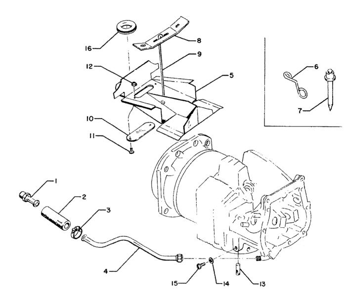
Figure 18 - Cylinder Head Drain Tubes and Intercylinder Cooling Baffles
