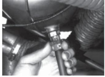
Take hold of the knurled nut and with a combination pushtwist motion, open the valve.
