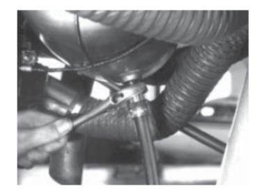
Simply remove the plug from the bottom of the oil sump and install the drain valve in the port. Wrench torque carefully. Safety wire valve to sump.
