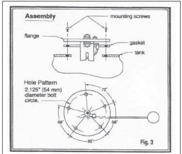
3. Slip the fuel sender assembly into the 2.322"(59mm) hole in the tank, turning assembly until it goes into the tank.
