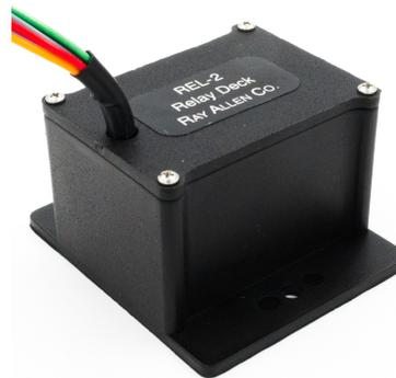
The REL-2 Relay Deck is designed to convert SPDT action switches into a DPDT action. The REL-2 will also drop both power white and gray power leads going to the actuator motor to ground. This motor braking function enables very precise actuator positioning. You will need one REL-2 per actuator.
