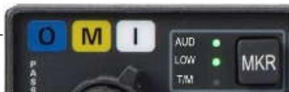
has an associated 400-Hertz 'dash' tone. The lamp and tone will be keyed at a rate of two tones/flashes per second when the aircraft is in the range of the Outer Marker Beacon.
