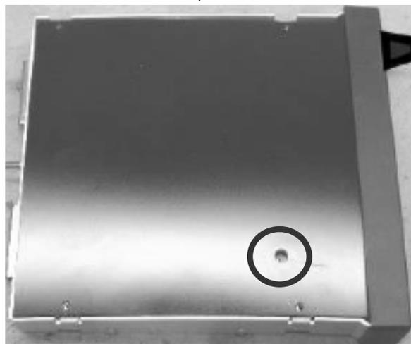
**Figure 2-4 – Unswitched 3 Audio Level (bottom cover removed)**
