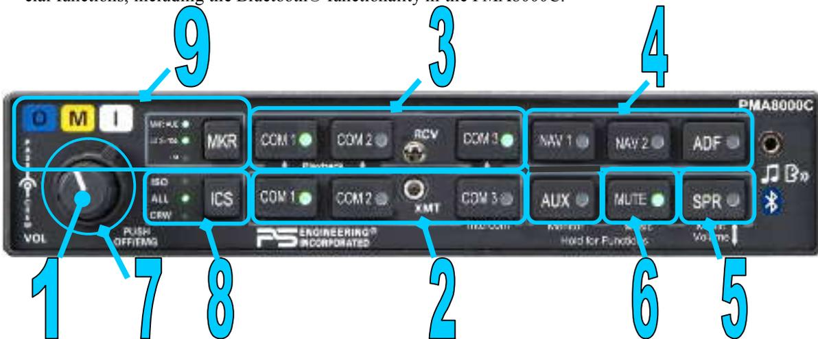
Figure 3-1 PMA8000C Operating Controls
