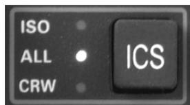
**ISO:** The pilot is isolated from the intercom and is connected only to the aircraft radio system. He hears the radios (and sidetone during radio transmissions). The copilot and passengers will hear the music sources as configured by the audio panel configuration Function keys. See page 11—Smart Function Keys for more details.
