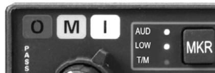
The Amber, **M**iddle Marker lamp is coupled with a 1300 Hertz tone, keyed alternately with short 'dot' and long 'dash' bursts at 95 combinations per minute.
