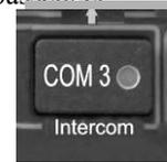
When in “*Alternate Intercom Function*,” the passengers will NEVER hear aircraft radios, even in the ALL mode. In addition, when in the ALL intercom mode, passengers will be able to converse with the crew, unless the aircraft radio becomes active, when the intercom audio from the passengers to the pilot and copilot is stopped, so the crew can focus on the radio. Passengers will always be able to talk to each other.
