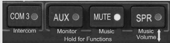
...tive, and the passengers never hear aircraft radios. Press and hold the COM 3 button until the audio annunciation starts (about 1 second) to activate the function, and you will hear “Alternate Intercom Function.” Hold the button again to exit, and you will hear “Standard Intercom Function.”
