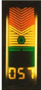
The AOA Pro Instrument's display is a four-color liquid crystal display that shall be located on the instrument panel or the glare shield.
