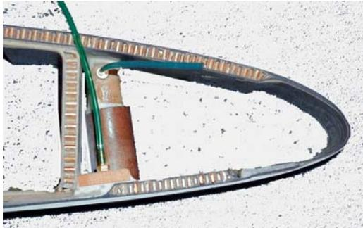
*Typical composite wing installation*
