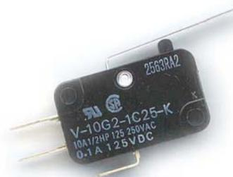
In some installations like RVs it may be easiest to activate the arm of the microswitch as the flaps move into the up position. In this case the AOA "FLAP" wire would be connected to the microswitch NC (normally closed) lug.
