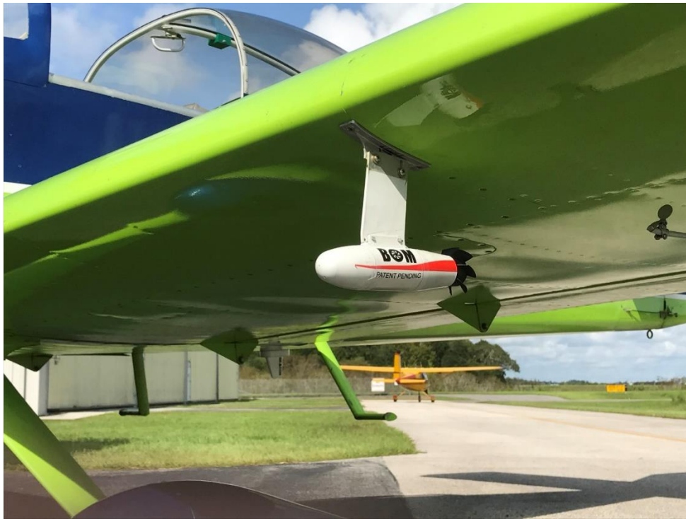
Fig 6. BOM installation on an RV9 using an external bracket. Notice the pitot on the right is at the same distance from the wing
