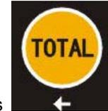
When the indicator show the last 4 digits, Press hold it, the indicator show "clr n", it means don't clear the total Weight, Press "Set" key to exit it; if you want to clear total weight, Press "ZERO" or "TARE" key, "clrn" change to "clry" it means clear total weight, then Press "Set" to clear the total weight and exit accumulating mode.
