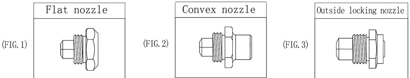
1: Flat nozzle (FIG. 1) is suitable for situations such as larger riveting plane space, larger rivet cap and shorter rivet rod etc.
