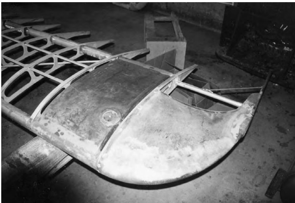
Fig 2-8. Just because you pick one type of construction, don't expect to escape working with other materials. This wing assembly features aluminum-tube spars, wooden ribs, and a fiberglass wingtip.
