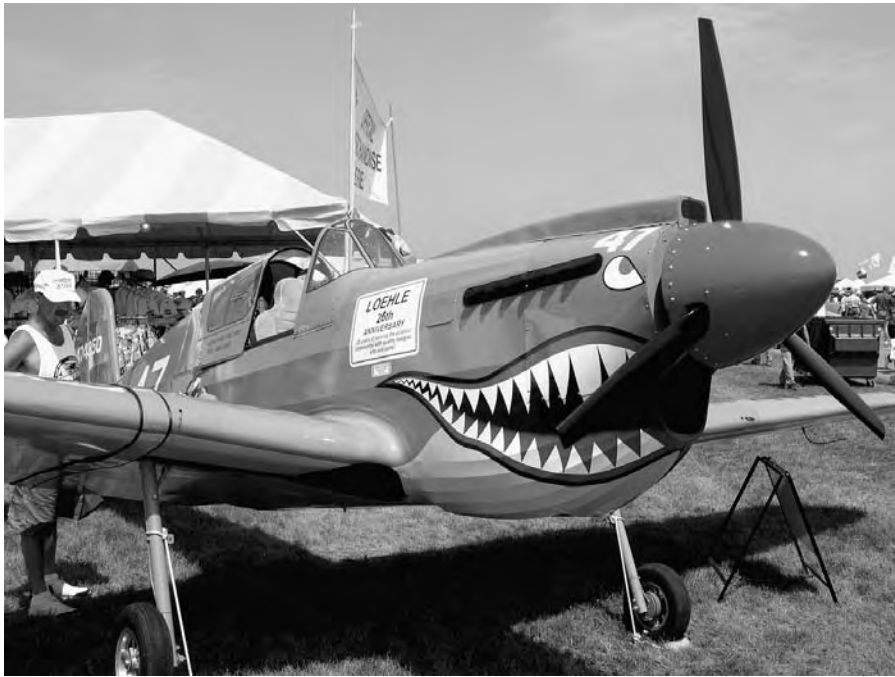
Fig 2-9. Many modern wooden kits, such as this Loehle P-40, feature prefabricated components and reduced construction time.
