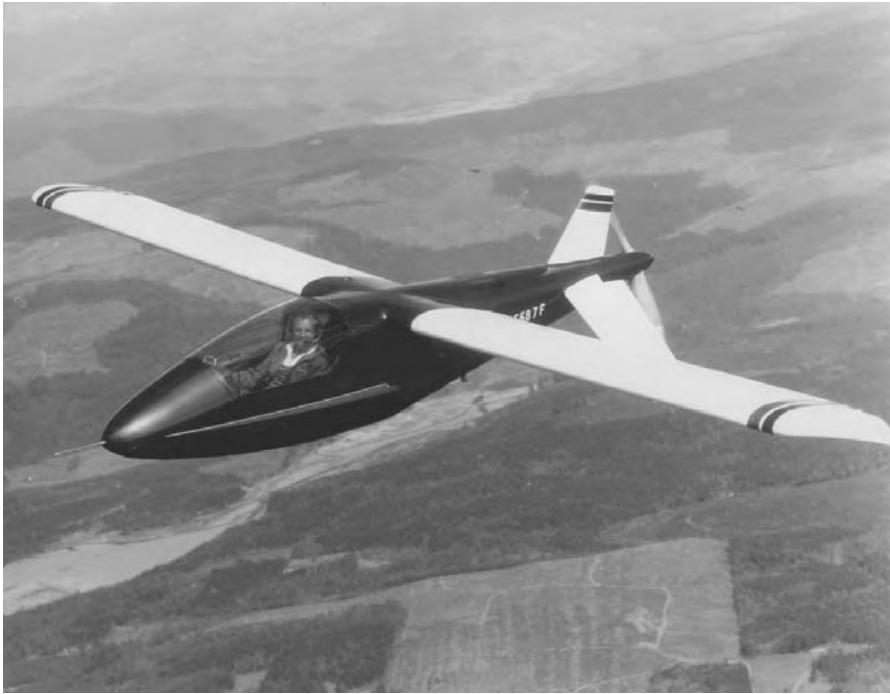
Fig. 2-7. The Mini-Imp uses a third method of composite construction, Taylor paper/glass.
