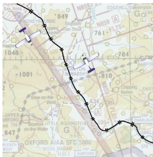
Figure 11.14 When following a line feature, fly to the right of the feature.
