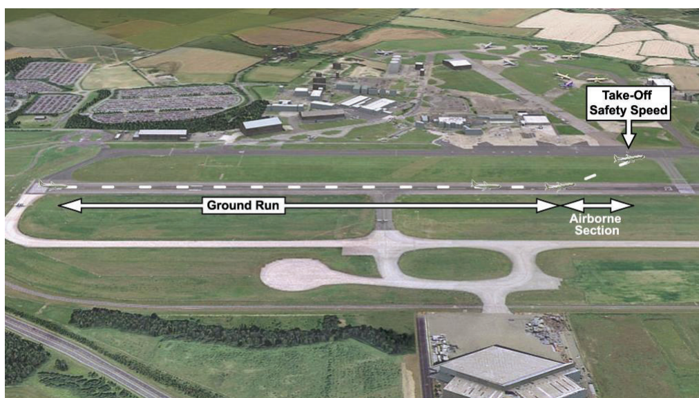
Figure 2.5: The take-off distance (TOD) is the total distance from brake release until the screen height.
