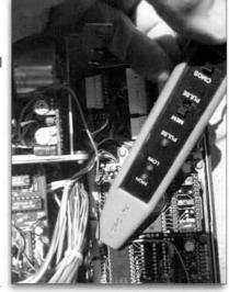
Logic probe to trace digital circuits.
