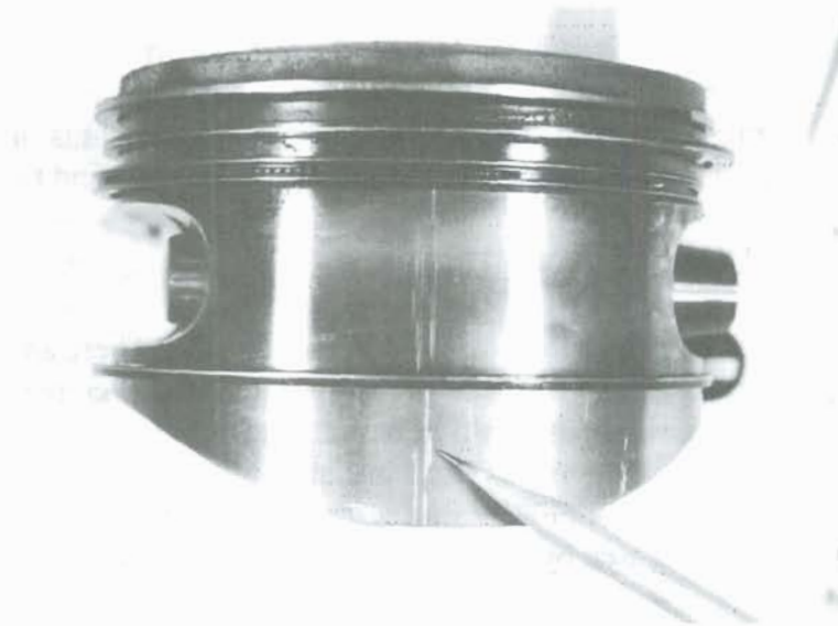
Figure 2-1 Piston skirt showing “comet” tracks from dirt particles.
