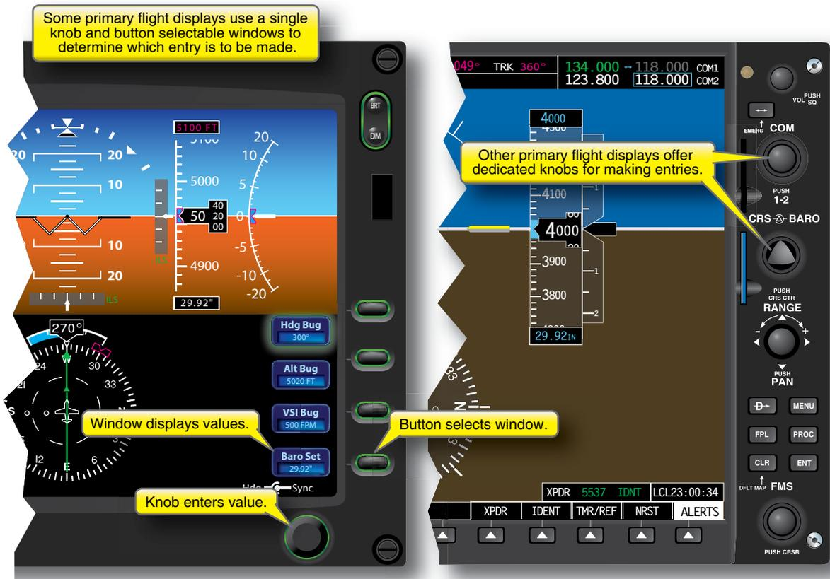
Figure 2-6. Making entries on a PFD.
