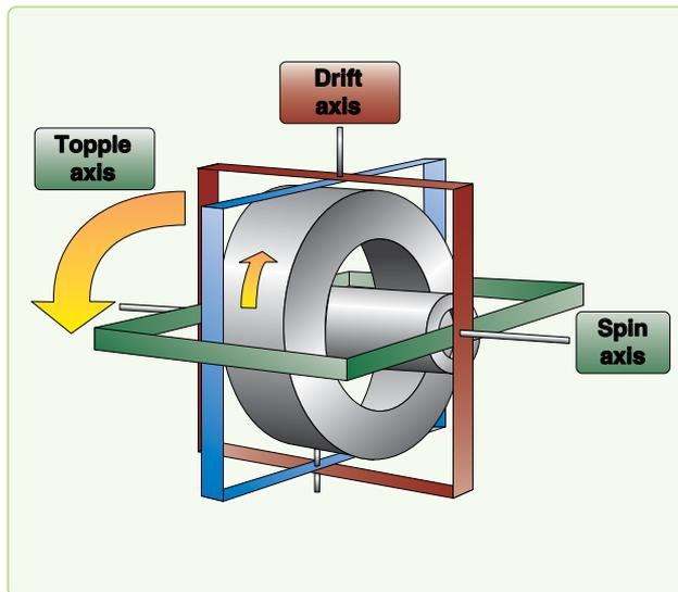
**Figure 3-9.** Gyroscope axes.
