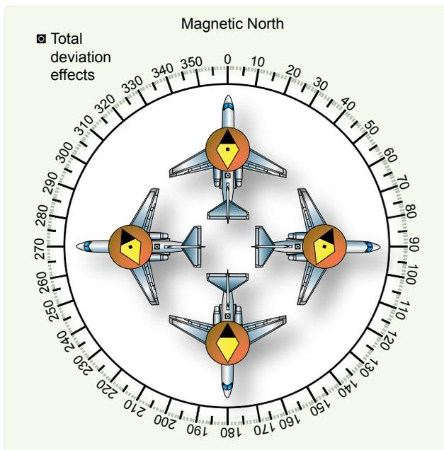
**Figure 3-6.** Deviation changes with heading.
