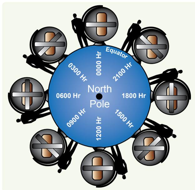
**Figure 3-10.** Apparent precession.
