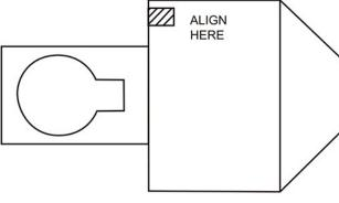
To lock, reverse above process after matching alignment symbol.
