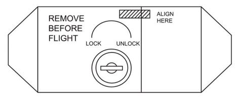
While holding PROLOCK with decal in legible position, insert key, turn clockwise, and pull.
