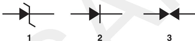
*Symbol 3 represents a current limiter. Current limiters are used primarily to sectionalize an aircraft circuit or bus.*
