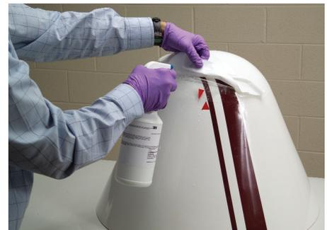
**Step 6:** Spray the radome/part and boot with 3M Application Solution. Then place the boot back on the radome (liner will be facing up). Using thumb nail, lift edge of liner from the boot to expose a small portion of adhesive. Spray 3M Application Solution on the adhesive. When removing the remainder of the liner, continuously spray 3M Application Solution on the exposed boot.
