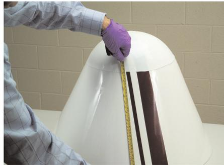
**Step 3:** Position the boot over the radome/part (adhesive/white liner side down against radome/part). Measure from the bottom of the boot and the base of the radome/part to ensure it is centered and properly positioned.
