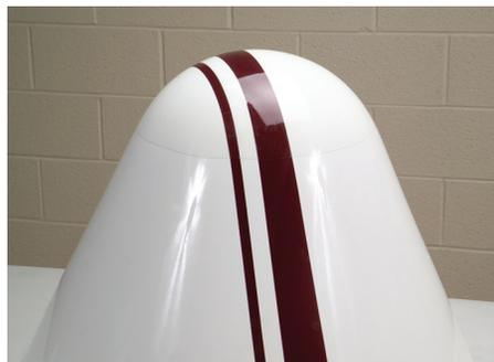
**Step 11:** Dry the surface of the boot with a clean cloth. If the boot is installed on an aircraft, allow to dwell one hour at 70°F (21°C) before flight.
