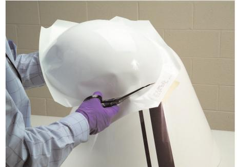
**Step 2:** Trim the boot with a pair of scissors about 1/4 inch above the trim line (trim line is located 1/2 inch above the base) that is found on most boots. Make clean, smooth cuts - avoid jagged edges.
