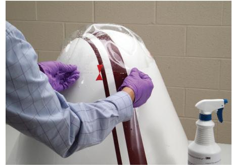
**Step 8:** Apply the boot to the radome/part taking care to match the index points at the top and sides of the boot. Reposition and reapply 3M Application Solution as needed until proper fit is achieved. Remove index marks.
