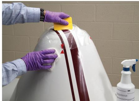
**Step 9:** Reapply 3M Application Solution to the outside of the boot. Starting at the center of the radome/part, use 1-2 inch strokes with the yellow squeegee to smooth out the boot - removing the trapped 3M Application Solution and air bubbles. Apply only light pressure to squeegee.
