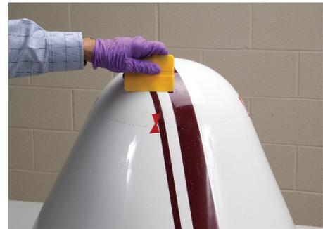
**Step 10:** Continue using short strokes working your way down to the base. If a bubble is trapped, carefully peel boot back, reapply 3M Application Solution and use yellow squeegee to re-adhere. Use a clean, lint-free, silicone-free cloth to absorb the liquid at the edges of the boot. This helps the edge of the boot to stay attached to the surface of the radome/part.
