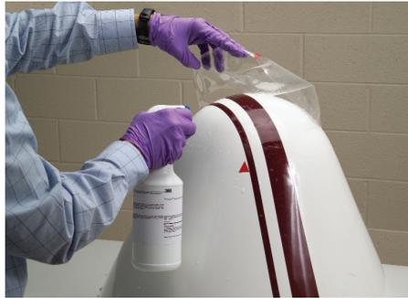
**Step 7:** Remove the 3M™ Polyurethane Protective Boot from the radome/part, turn inside out again. The adhesive side should be facing the radome/part. Heavily spray radome/part and boot with 3M™ Protective Tape Application Solution allowing for easy repositioning. The more 3M Application Solution used, the easier the application will be.
