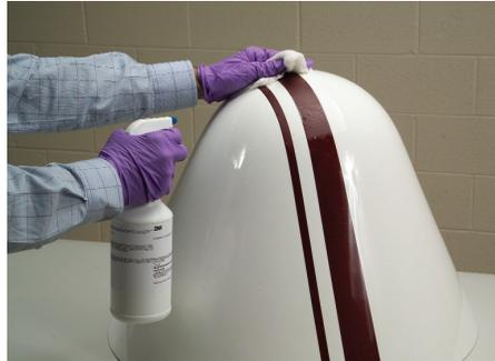
**Step 1:** Make sure hands are clean and free of oils and grease. Clean the radome/part and the boot (top side and bottom side) with 3M™ Protective Tape Application Solution to remove the corn starch. This will ensure maximum adhesion.
