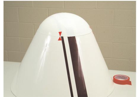
**Step 4:** Use 3M™ Vinyl Tape 471 to mark three index points on the radome/part (one on the top and two on the sides approximately 90° apart) clearly establishing the center point, so the boot can be repositioned properly. Then mark three additional index points on the boot opposite of marks currently in place.
