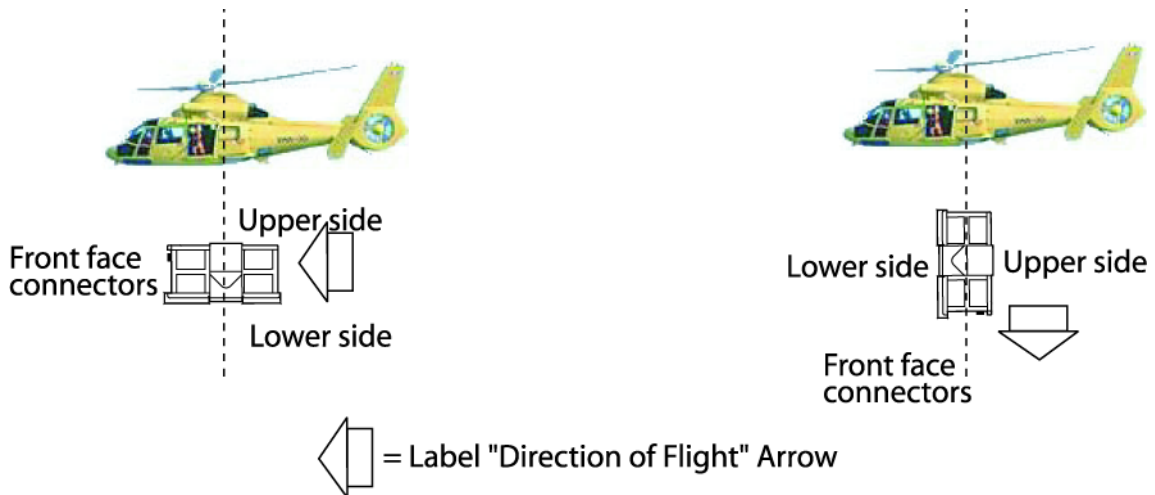
Figure 204: KANNAD 406 AF-H installation
