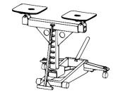
**Belly pads**: Center the "T" stand (arrow) below the aircraft's longitudinal centerline and extend slide tubes equally to place pads equally inboard between landing gear legs roughly 1-2 inches from where the legs enter the fuselage and aligned directly under the gear box structure.
