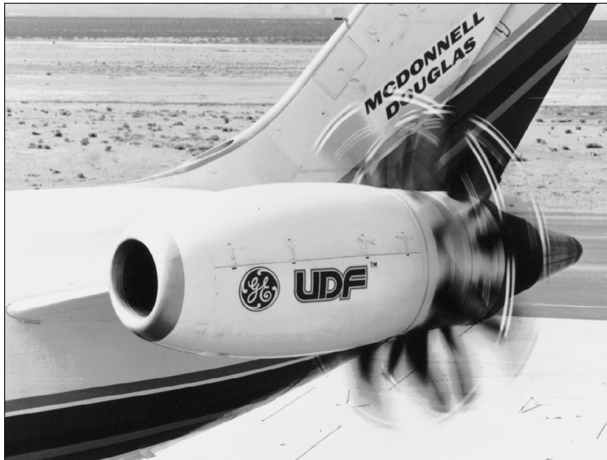
Figure 1-5. The Unducted Fan™ engine is an ultra-high-bypass turbine engine that promises quiet operation with low fuel consumption at a speed higher than that used by turboprop-powered aircraft.
