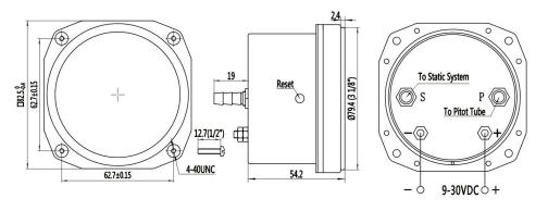
Airspeed indicator scale drawing
