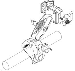
Tighten the 3.75" shaft to secure your desired position
