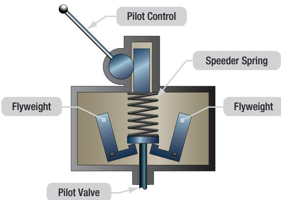
Figure 17-22. Governor sensing an overspeed condition.
