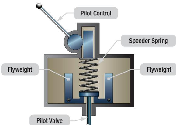
Figure 17-23. Governor sensing an on-speed condition.
