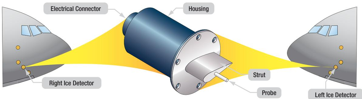
Figure 12-4. An ice detection probe on large aircraft warns the flight crew of the presence of ice.
