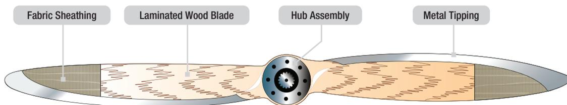
Figure 17-24. Fixed-pitch wood propeller assembly.
