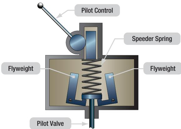
Figure 17-21. Governor sensing an underspeed condition.
