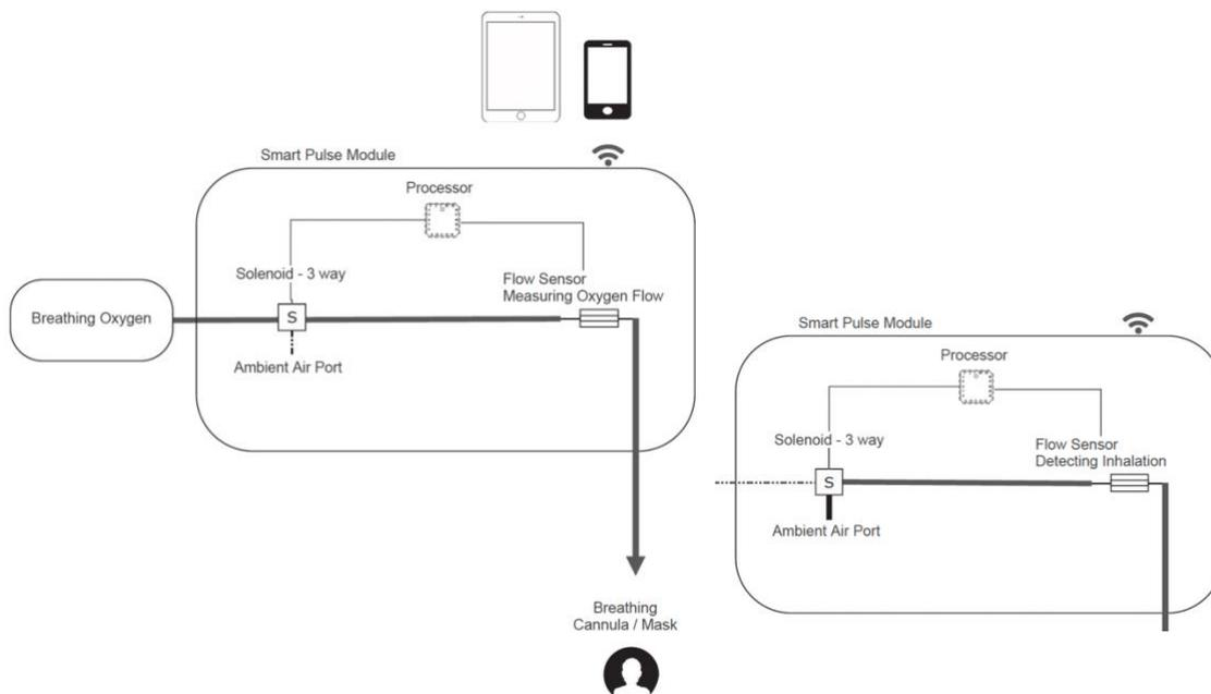
All of the AVI smart oxygen systems – portable and built-in – are built upon an innovative and patent pending arrangement of an optical flow sensor and a low wattage high pressure 3-way solenoid valve. The optical flow sensor enables very sensitive long-range detection of breathing combined with measurements of oxygen flow, while the 3-way solenoid provides a 20ms bursts of oxygen switched with breathing detection mode.
