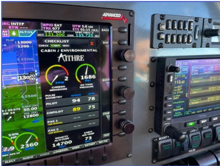
While the RS-232 data stream provides more fields, the AVI EX series also includes a discrete 12V fault line that is driven low to ground when the pilot is not breathing or when oxygen pressure is absent. This discrete fault line is supported by many modern avionics systems and can often be configured to throw a warning flag within the EFIS.
