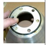
Insert hub bolt and lock washer through the front side of the rim half (The half with the valve stem) and O-Ring spacer plate
