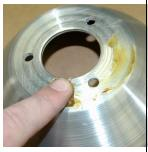
Grease to the O-Ring and align the spacer plate with the holes in the rim
