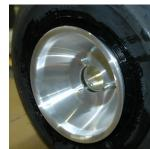
Tighten the bolts to the hub attach the flange nuts to the excess thread protruding form the back of the hub to secure the hub bolts for safety.
