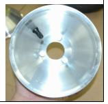
Apply soapy water to both sides of the tire bead and insert front half and back half of the rim together using the 3 hub bolts. Insert hub bolts from the valve stem side.
