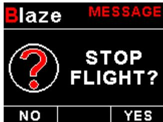
Press the F1/Up button during the normal display mode to manually start/stop a flight. This key is only active if the MAP-4 is setup to select the manual flight option under the "TIMERS" setup menu.
