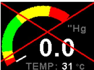
The red cross over the display means the MAP-4 has lost communications with the external RDAC unit. Check the wiring between the MAP-4 instrument and the RDAC unit. This error message is only available when the external RDAC is selected as the data source.
