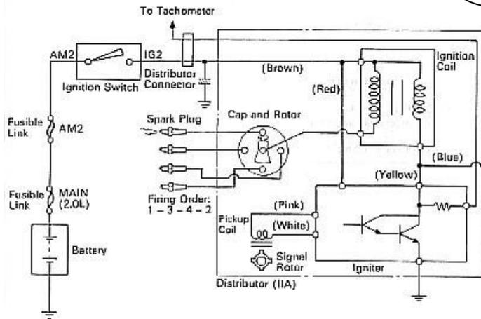
Connect rev counter input of MAP-4 to this line. Ensure you have a connection from the MAP-4 ground to the engine block.
