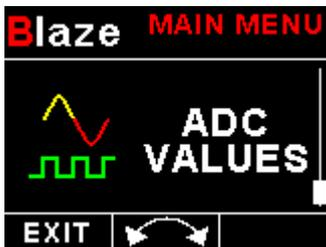
This menu displays the ADC values that have been read from the pressure and temperature sensor.
