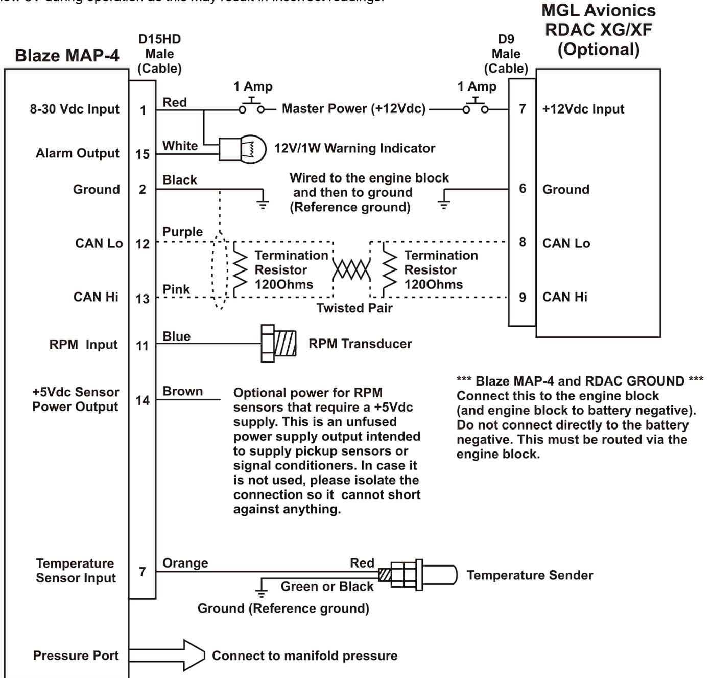
**Please note:** The +5V Sensor power output line is unprotected and intended only for the supply of a hall-effect, optical or gear tooth sensors. Connecting any voltages (such as the 12V supply) to this line could destroy the instrument. The +5V line may supply currents of up to 50mA. Should your sensor require greater currents you must supply it from another source.
