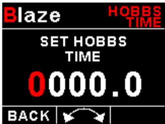
This function allows you to set the engine Hobbs meter to any value. Typically, you would use this function to set the Hobbs meter to the current known engine time. Use the rotary control to change the value. Press the rotary control to accept and exit the menu option. If the Hobbs code is set to another value beside zero, then the pilot will be prompted to enter the Hobbs access code before allowing him to change the Hobbs time. This feature is useful for chartered and flying school planes.
