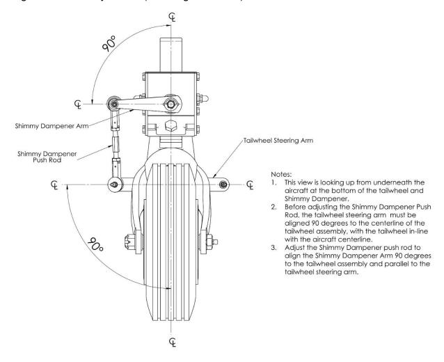
After the shimmy dampener pushrod assembly is properly adjusted, cycle your tailwheel assembly around both directions to ensure that the pushrod assembly does not bind and that the tailwheel steering arms break away properly. After checking this, tighten both push rod jam nuts against the rod end bearings to ensure they do not move over time.
