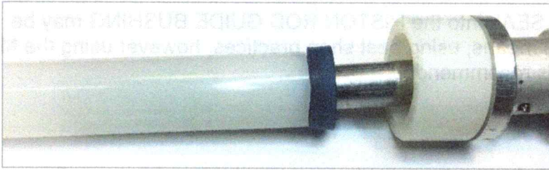
FIGURE 4 – PUSH TUBE, used to push LIP SEAL onto piston rod and into compression ring into PISTON ROD GUIDE BUSHING.
