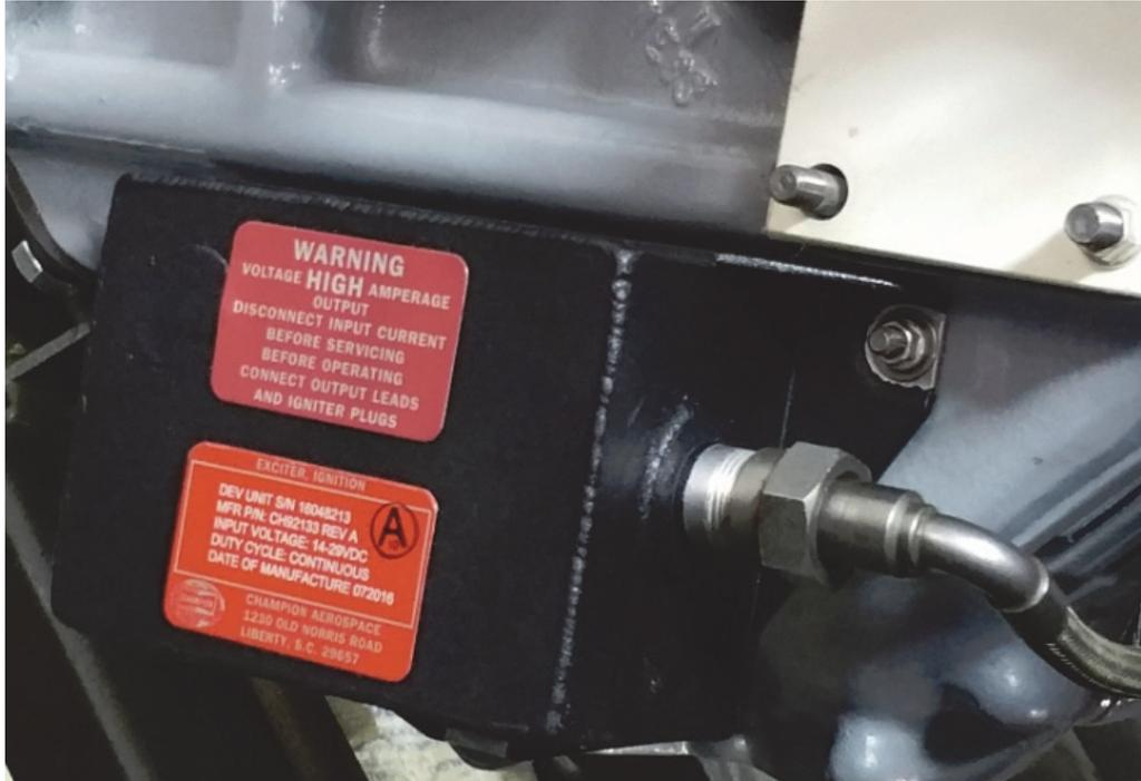
The Champion Aerospace Ignition Exciter Assembly, Model CH92133 is eligible by **FAA-PMA** for use on the Rolls-Royce Model 250 Series I, II, III & IV turbine engines as approved for replacement of the following exciter models:
