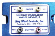
Advanced regulator/rectifier circuit provides steady 13.8 volt output regardless of load. Maximum output 220 watts, 16 amps. Accepts AC input from 15 to 100 volts. Can be used with AC strobe.
