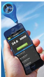
The WeatherFlow Wind Meter is an anemometer that fits in your pocket. It's the first hardware product we have created for the general wind- & weather-addicted community.
