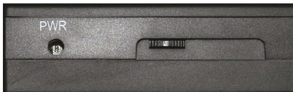
Figure 14 - D1 Right Side (left to right): PWR Port, Rocker
