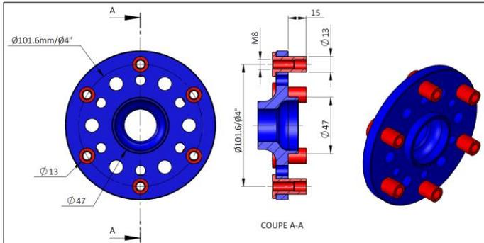
**JABIRU 2200 engine propeller-shaft**
