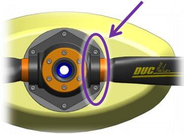
Once the desired pitch angle obtained, slightly tighten the **assembly screws of the hub**, those around the foot blade and then perform the same operation on each of the other blades.
