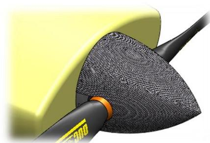
After a final verification (position and orientation of parts, tightening...), mount the spinner on the mounting plate by **tightening the spinner screws to a torque of 4Nm (0.4kg/m)** with the appropriate tools.
