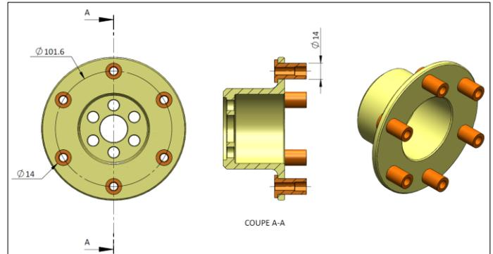
**UL Power engine propeller-shaft**
