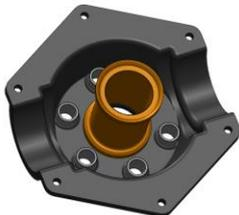
Place the hub spacer in the center of the rear half-hub.
