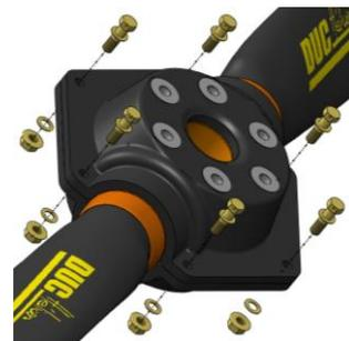
From the front hub, set up the 6 screws and washers for hub assembly. At the rear, place washers and lock nuts.
