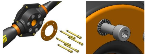
Place the hub clamping washer on the front of the propeller hub (side logo).
