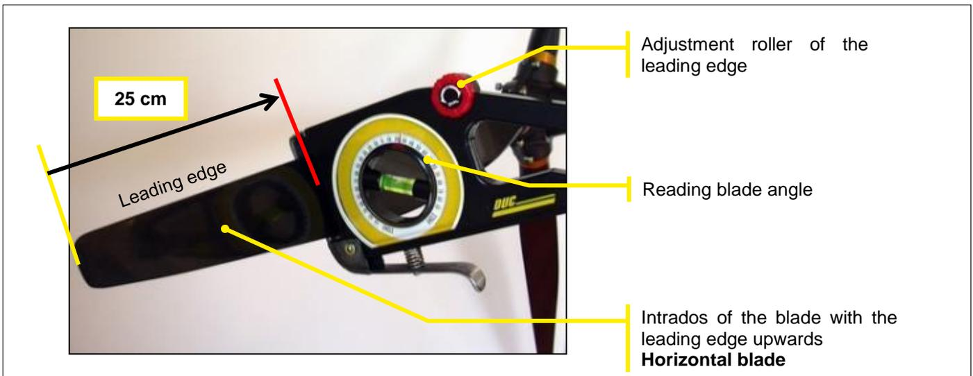
Horizontal blade, leading edge upward, place the adjustment tool at 25 cm from the tip of the blade, intrados side (flat), handle down.
