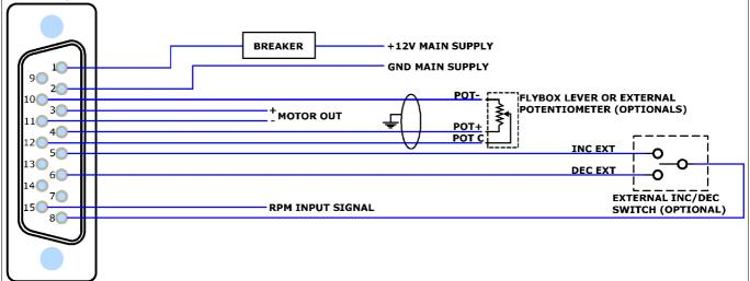
15-pole female connector, view from wiring side
