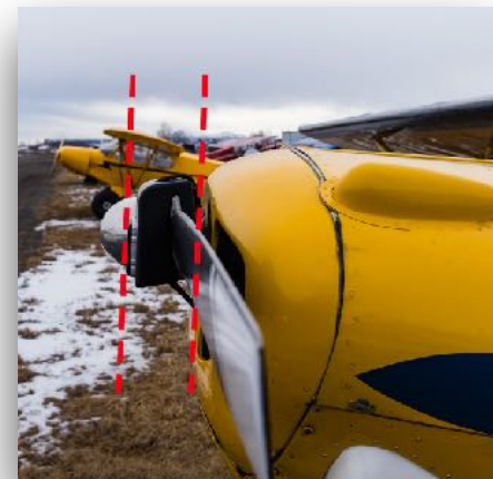
Face of Inclinometer parallel to Crankshaft Flange
